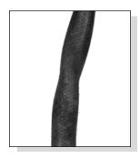
Partly collapsed inlet line shown.
