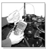
Testing the temperature at the discharge fitting.
