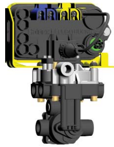
PLC Select FFABS (2 Service Delivery Ports)
