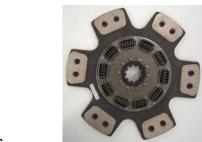
DCF-CO MU128925-103 Spline 2" 10 MU128925-45\* SS108925-25\* Buttons 6 Ceramic
