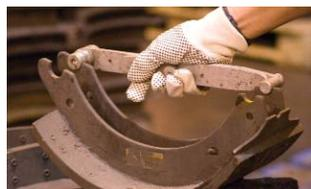
Shoe quality begins at core check-in. Out of spec shoes are scrapped.
