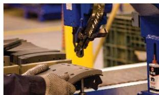
Rivet torque specifications are critically maintained to ensure reliable lining to shoe attachment.
