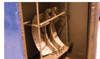
Individual shot blasting ensures 100% removal of external contaminants - necessary for reliable coating coverage.
