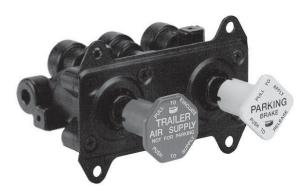
The Bendix<sup>®</sup> MV-3<sup>®</sup> dash control module is a twobutton, push-pull control valve housed in a single body which includes a dual circuit supply valve and a check valve. The MV-3<sup>®</sup> valve can duplicate the functions of any existing two or three valve push-pull system and has the advantage of reduced plumbing.
